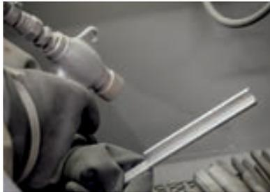
Similarly, the flute of the tool is cleaned with a formed abrasive wheel and then polished with a fine abrasive compound to remove any marks left by the previous process, creating a fully polished flute.
